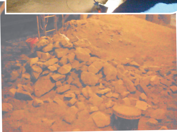
Rock hard cement removed from silo to facilitate flow.
