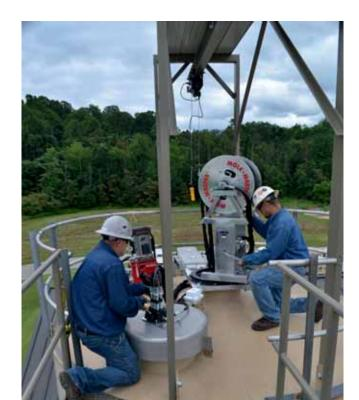
Junior<sup>™</sup> is easy to transport and assemble. The hose reel is independent from the boom assembly which allows for easier set-up in close quarters.
